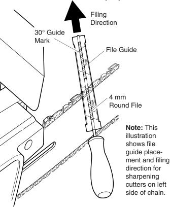
Figure 20 - File and File Guide Placement On Chain
